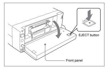
**2** Press the EJECT button while the AC adaptor or battery is attached to the unit.
